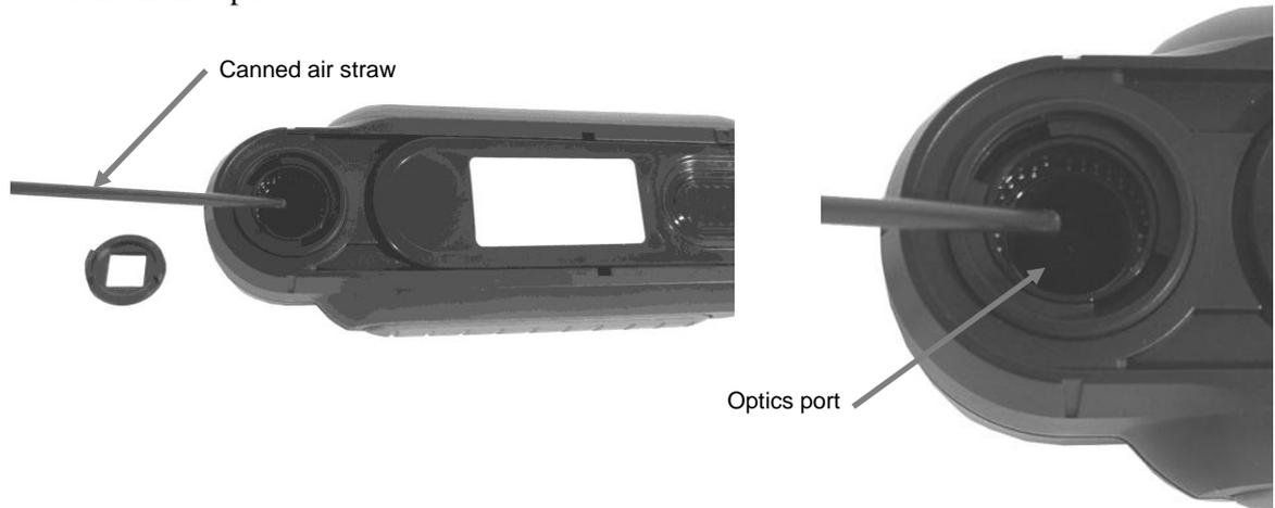
4. Reposition the aperture over the optics housing and turn 45° clockwise to lock into place.
